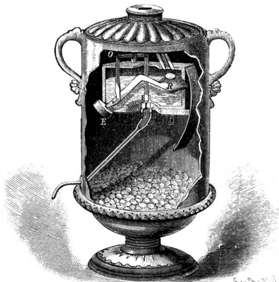
Fig. 2.—NOBLE'S AUTOMATIC PERFUME DISTRIBUTOR. PATENTED IN 1889.
