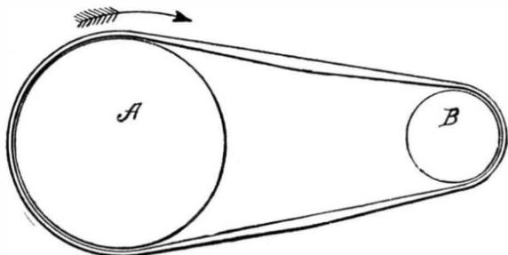
100 revolutions per minute, driving with a belt a pulley 12 inches diameter, 300 revolutions.
