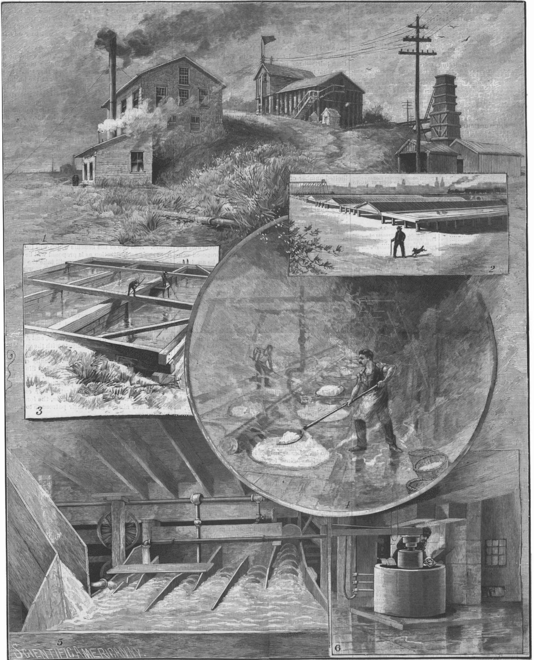
1. New York State pumping station and reservoir. 2. Solar evaporation. 3. Settling vats. 4. Salt boiling in kettles. 5. Washing salt. 6. Centrifugal drier,
