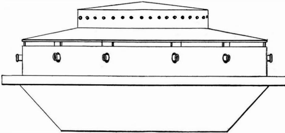
to the body of the battery, by sails raised on its exterior parts, or by manual application. In this last way it may be effected by men in the hold, drawing on a lever fastened to a post fixed to the keel, and rising through a well-hole in the center of the battery. The strength of horses might perhaps be applied to the same purpose. The cables by which the keel is held are to be entirely under water and thus secure from an enemy's shot.
