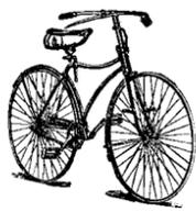
\$85 Lovell Diamond Safety \$85 Diamond Frame, Steel Drop Forgings, Steel Tubing, Adjustable Ball Bearings to all Running Parts, including Pedals, Suspension Saddle, Finest material money can buy. Finished in enamel and nickel. Strictly high grade in every particular. No better machine made at any price. BICYCLE CATALOGUE FREE. JOHN P. LOVELL ARMS CO., 147 Washington Street, BOSTON, MASS.
