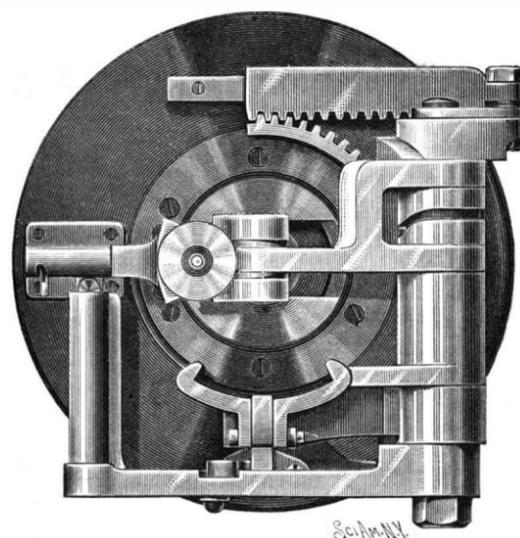
Fig. 3.—MODIFIED MECHANISM—REAR VIEW OF BREECH CLOSED.
