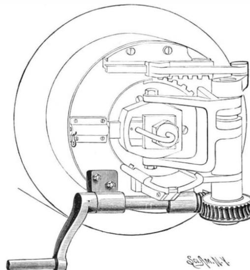
Fig. 8.—GEARING USED ON GUNS OF LARGE CALIBER TO WORK MECHANISM.
