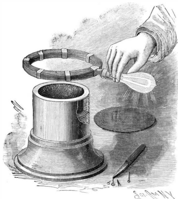
Fig. 7.—EXPERIMENT WITH A WATCH DEMAGNETIZER.
