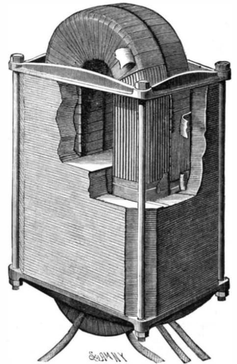
Fig. 2.—DETAIL OF CONVERTER.
