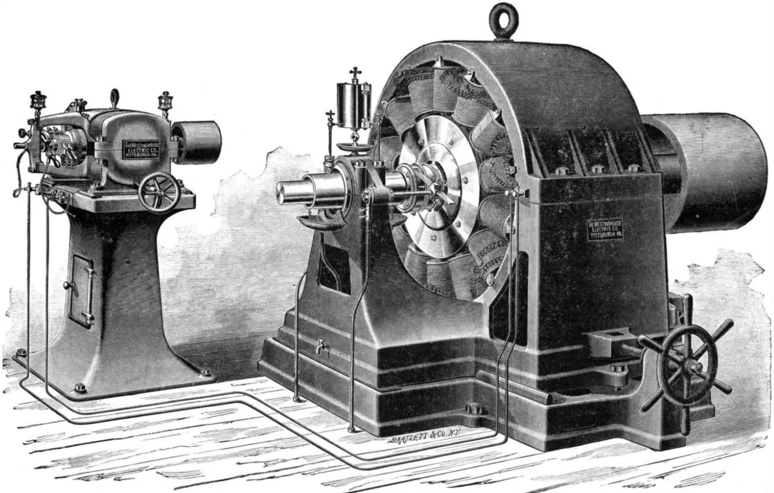
Fig. 3.—WESTINGHOUSE DYNAMO AND EXCITER—1500 CANDLE POWER.
