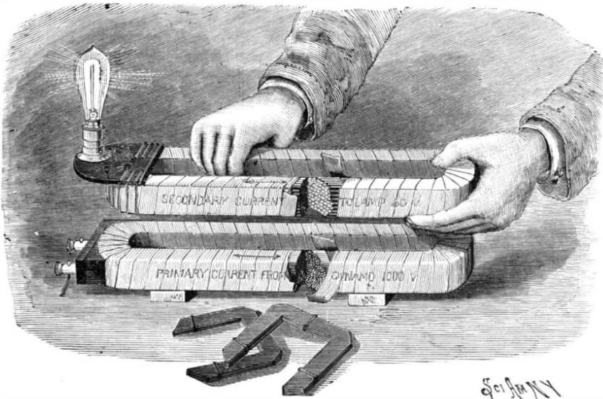
Fig. 4.—EXPERIMENT SHOWING PRINCIPLE OF CONVERTER.
