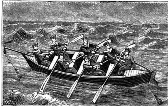
Fig. 2.—LIFE-BOAT WITH OIL BAG.
