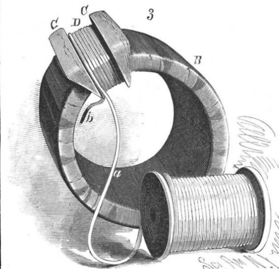
Fig. 3.—WINDING THE ARMATURE.
