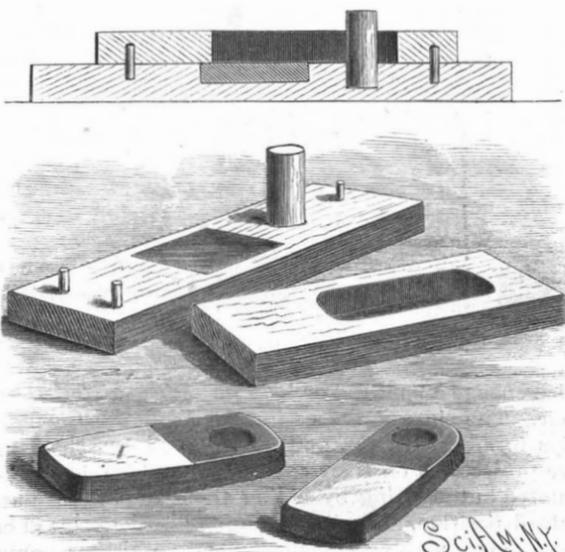
LEAD COHESION BLOCKS—THE MOULD.
