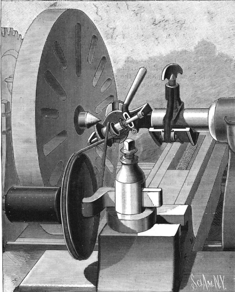
**RANDALL'S LATHE CENTER GRINDING MACHINE.**
