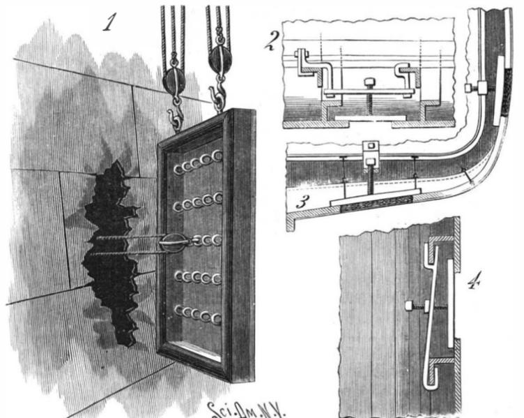
**SPEIRS' APPARATUS FOR CLOSING APERTURES IN HULLS OF VESSELS.**
