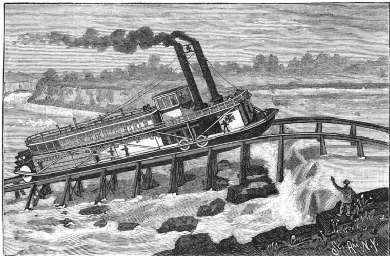
GRONDAHL'S APPARATUS FOR CARRYING VESSELS OVER OBSTRUCTIONS.
