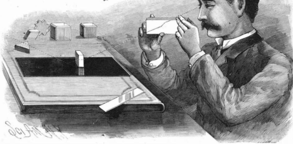
By turning the analyzing plate on the axis of the light beam, some curious effects may be observed. When the plates are at right angles with each other, the polarized beam will be nearly quenched,\* and when they are parallel with each other the reflection of the sky will be quite bright.
