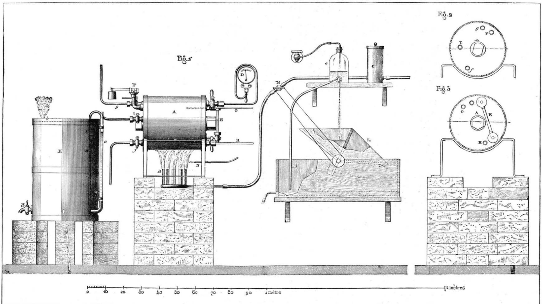
Fig. 1.—General Arrangement of Boiler and Accessories. Fig. 2.—Elevation of Boiler Front. Fig. 3.—Elevation of Rear End.
