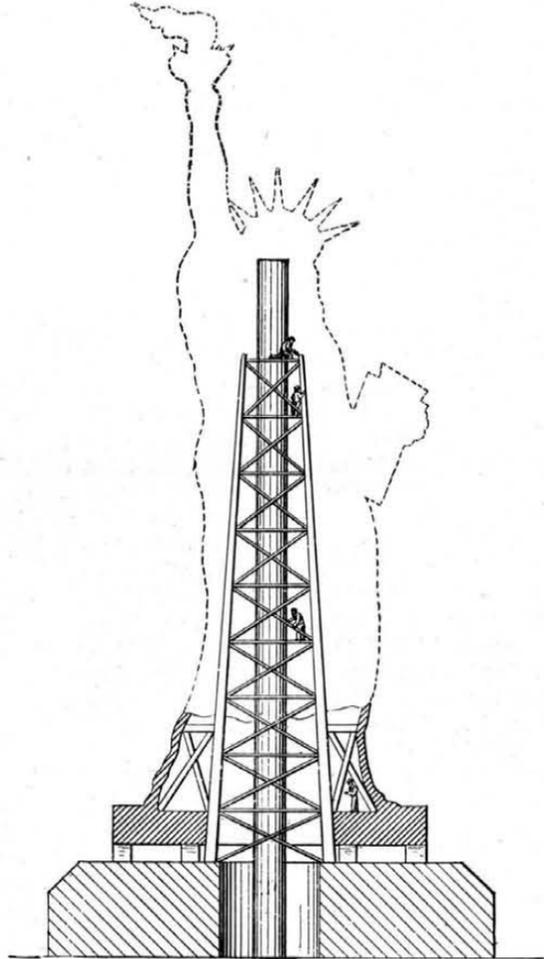
Fig. 2.—INTERIOR BRACING AND FRAME.
