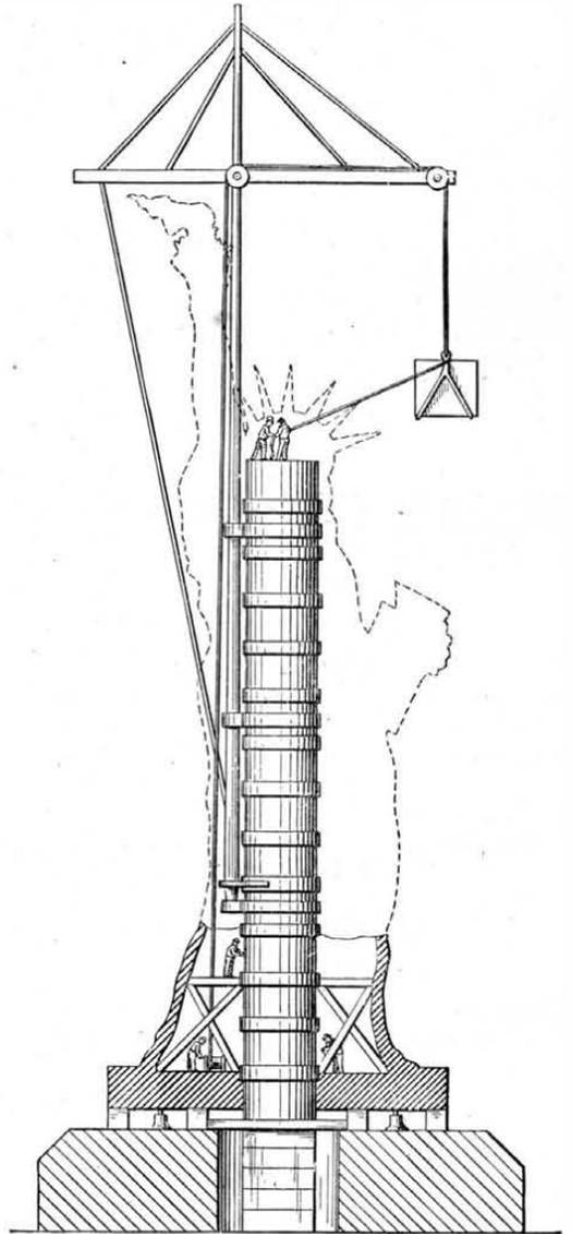
Fig. 1.—MODE OF SETTING UP THE STATUE, CRANE, INTERIOR TUBE, AND BRACING.
