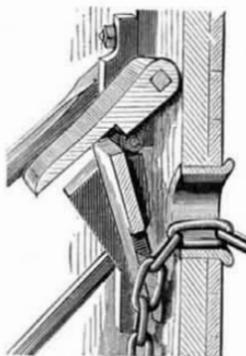
of a vessel, and is further strengthened by stay rods which are to extend to the deck. When the door is shut down it engages the chain, and when it is opened by means of the lever it releases the chain.
