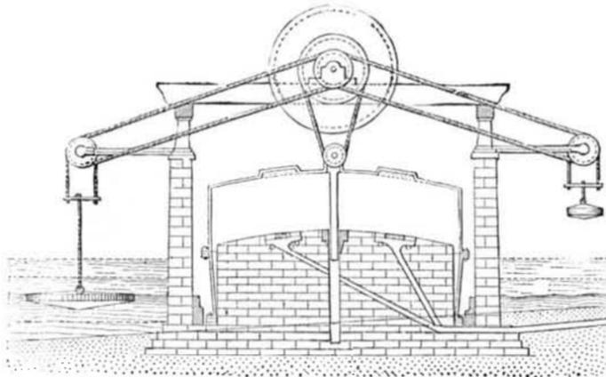
Fig. 1.—Float and Iron Compressing Bell.
