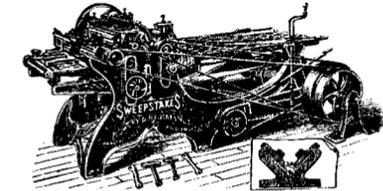
SWEETSTAKES, WITH THE ELLIS Patent Journal Box. The best Planer and Matcher ever made. Planing 20 in wide, 6 in. thick, weight 2,300 lbs., \$300; planing 24 in wide, 6 in. thick, weight 2,600 lbs., \$350. Beading, Arbor and Head, extra, \$20. Sash, Door, and Blind Machinery a specialty. Send for descriptive catalogue to Rowley & Hermance, Williamsport, Pa.
