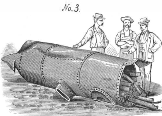
part (see Fig. 1) which was blown to pieces. The original form of this part is shown in dim outline, while the external sheet, with the screw stays attached, is seen spread out in the act of commencing its flight to parts unknown. Up to this time this plate has not been found.
