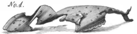
surface in case of low water in the boiler; but there was unmistakable evidence that the so called safety valve was and had been for some time absolutely inoperative. The iron stem of the valve was immovably fixed by corrosion in the iron bonnet of the valve case. This valve, which is of the wing pattern, is 2½ inches diameter, was loaded by lever and weight to blow off at about 60 pounds when in order.
