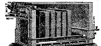
It does prevent, check, warp or hardened surface, involving the true principle of seasoning, extracting the moisture from the center by suction, rapid circulation of air, with moderate heat; thus securing the cheapest dry room in construction, quickest in operation, and the most perfect in results. Address
