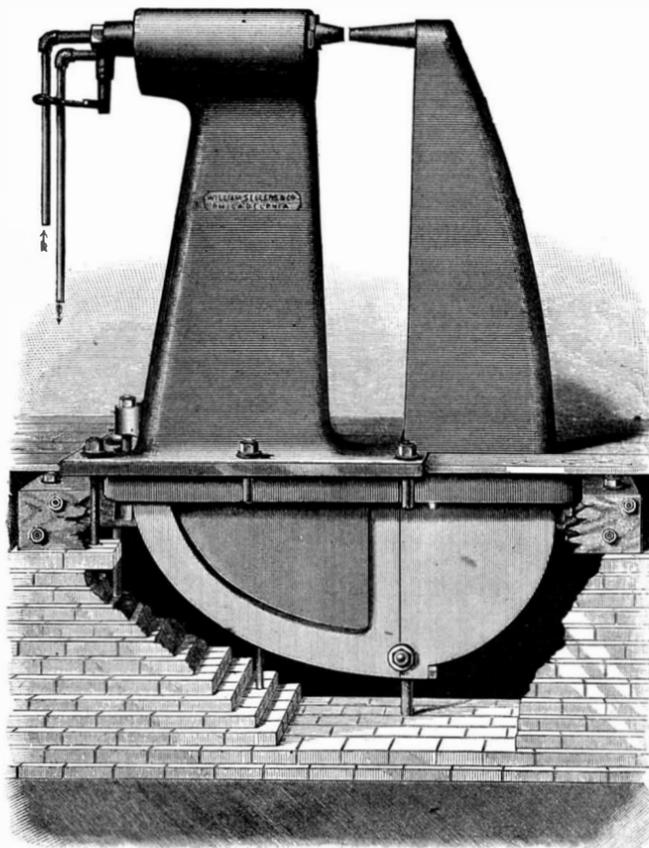
Fig. 4.—STATIONARY RIVETING MACHINE.
