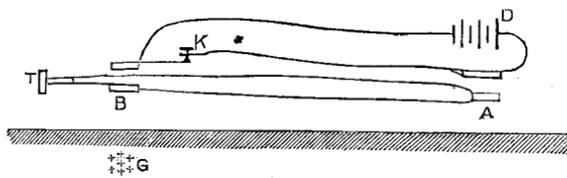
would be to keep one pan of the balance stationary in one place, while the other was being moved about so as to feel for the hidden ores. The latter method is shown in the accompanying sketch, where A is the stationary pan of the balance, and B is the movable pan carried by the prospector; C is a metal lode under the surface, D is the battery, and K is the key in the primary circuit of the balance, and T is the telephone in the secondary circuit.
