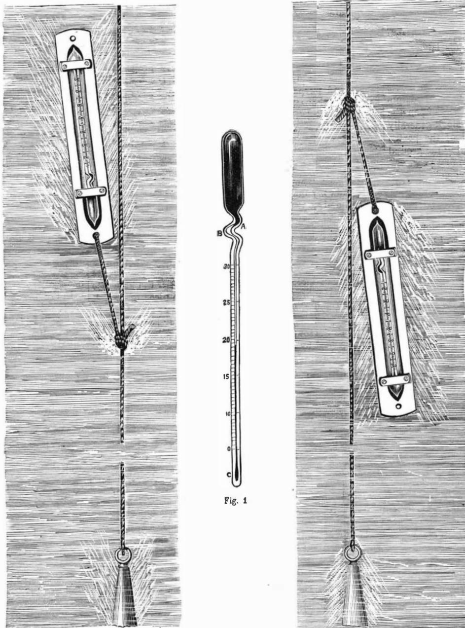
**NEW THERMOMETER FOR OBTAINING THE TEMPERATURE OF THE OCEAN AT GREAT DEPTHS.**
