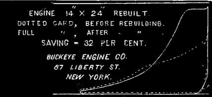
The above is reduced from an actual diagram. THE BUCKEYE AUTOMATIC CUT-OFF fitted to Throttling Engines at moderate cost. Increased power, high economy, absolute regulation guaranteed. Estimates furnished on description. BUCKEYE ENGINE CO., 87 Liberty St., New York.
