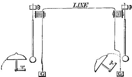
phragm. The action of the apparatus will readily be understood from the engraving, where a wire in the form of the letter U is shown, with the bend attached to the diaphragm, and its ends dipping into the separate cells, and thus made to form part of the circuit when the line is joined to the instrument at a and c.
