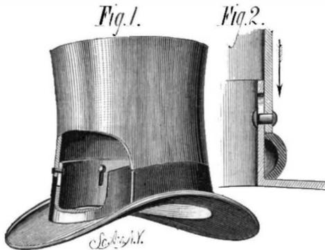
fitted to the head. The body slides on the rim portion as shown in section, Fig. 2, and is guided by slots and pins, and supported by a cushioning spring. This device was patented through the Scientific American Patent Agency, February 26, 1878, by Mr. José M. de Celis, of New York city.
