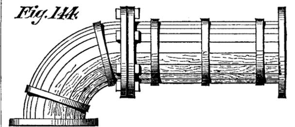
ber of tiers is discretionary; but it is well to have the top piece comparatively thick, so that it shall not be liable to curl, as it would be apt to do if the turning left it thin. If the joints of the tiers are well surfaced and well glued, neither nails nor screws will be needed. It is not compulsory to make each layer a continuous piece, and it will save stuff to make every alternate layer of two pieces; but the bottom and top layers are better if each be made in one piece.
