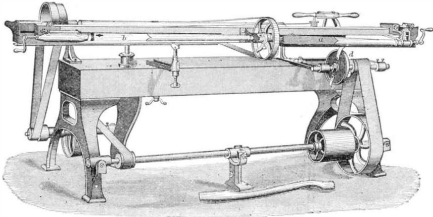
then turned over, and the other side similarly dressed. On drawing the spoke forward and releasing it from the stop, the desired bevel is given to the edge of the tenon by means of the cutters, the particular inclination being determined by an adjustable angle gauge.
