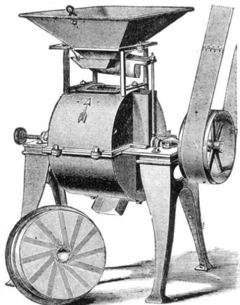
in order that a high speed may be obtained. It is a French burr mill and corn cob breaker combined; it will remain true in line while shaving both sides of tender bran between the millstones; it has journal boxes with caps to take up wear; it is simple in design; and finally, the millstones may be easily removed and dressed.
