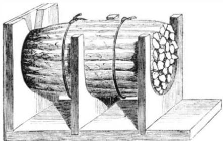
upright boards. When the frame is nearly full, the shoots are passed in through the wedge-shaped opening shown. Fig. 3 shows the same buncher when filled.
