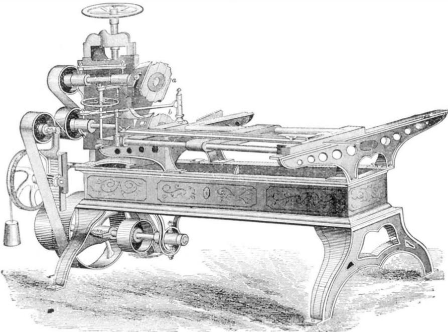
point of the hub rests on a block keyed up by wedges. The butt of the hub rests on a pivoted bar whose carriage is vertically adjustable on the standard by a lever and rod in the rear. The mandrel bolt clamps the pivoted hub rest to a bar on the back of the standard.
