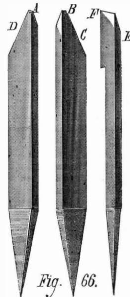
The temper of all these tools should be drawn to a light brown color, and the instruction given for grinding bench tools should be rigidly observed in grinding and oilstoning these turning tools.
