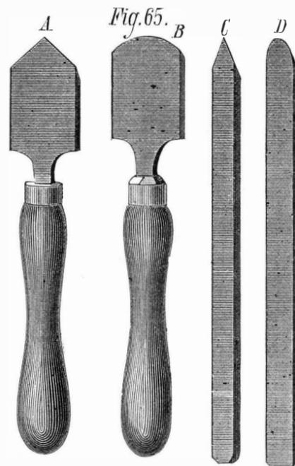
quence, it is less liable to cause the work to jar or tremble. It is usually made about 2 feet long, which enables the operator to hold it very firmly and steadily. It is used with its top face lying horizontally, and should be kept keen. D, in the same figure, represents a similar tool, with a round nose; this latter is not, however, made long, and may be used in a handle.
