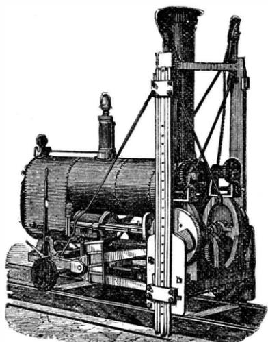
WARDWELL PATENT, FOR CUTTING STONE INTO VARIOUS SIZES AND DIMENSIONS IN ALL KINDS OF QUARRIES. STEAM STONE CUTTER CO., RUTLAND, VT. SOLE PROPRIETORS AND MANUFACTURERS. Three Machines at Philadelphia Exhibition, in Annex No. 2, Machinery Hall.
