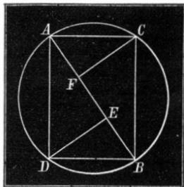
To cut the best beam from a log, divide the diameter, *ab*, into 3 equal parts, *af*, *fe*, and *eb*; and from *e* and *f*, draw the lines *fe*, *ed*, at right angles to *ab*. Join *ac*, *rd*, *bc*, and *bd*; then *abcd* is the strongest beam.
