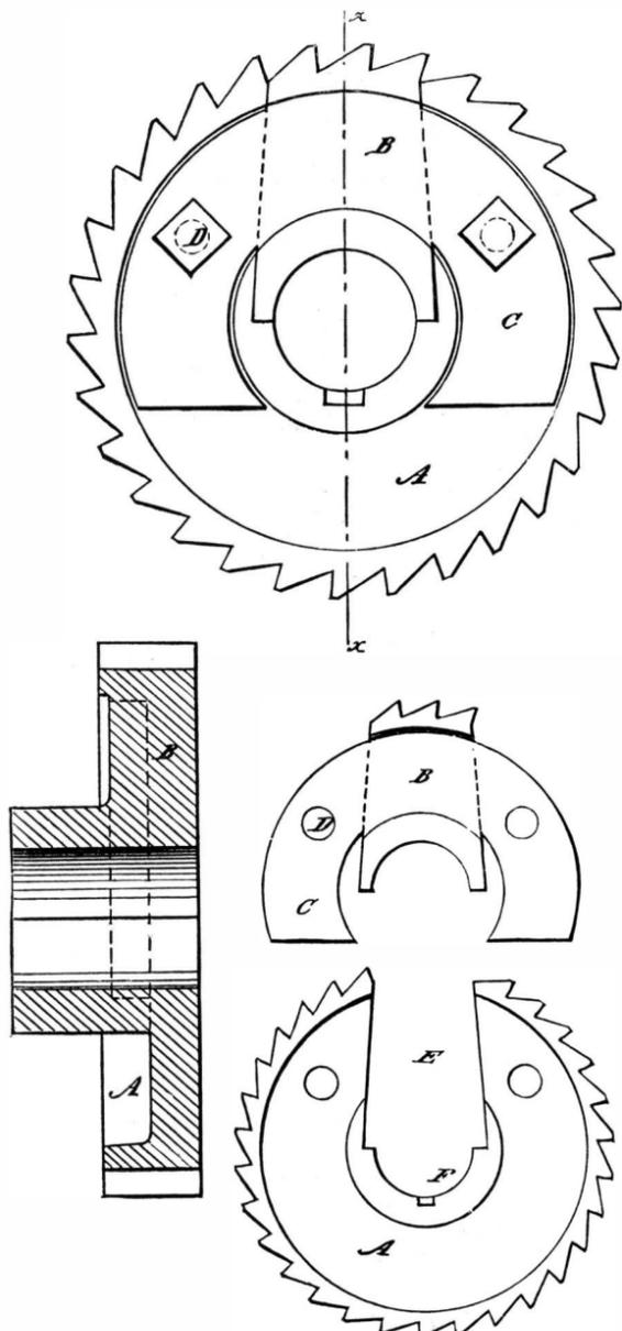
tail shape, so that the part, B, will be securely held against the expanding effect of the key, by which the wheel is secured to the shaft.
