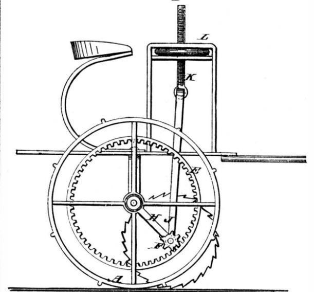
sired, or as the character of the land to be operated upon may require. To the center of the bail, attached to the saw shaft, is pivoted the end of a screw, K, which passes up through a hand nut, L, swiveled to a bracket, attached to the frame, so that, by turning the said hand nut, the saws may be adjusted to enter the ground to any desired depth, or may be raised from the ground. The axle is suitably bent to accommodate the saws.
