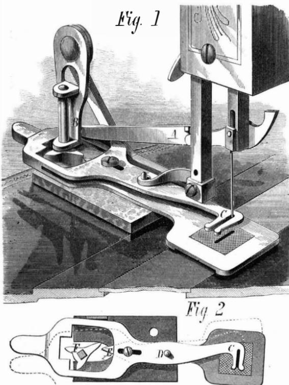
It is obvious that, in order to give a button the necessary movement under the needle so that the latter can pass backward and forward from hole to hole, a different feed motion from that usually found in sewing machines is needed. And, moreover, such motion must be adjustable according to the distance between the holes in the button. This seems to be neatly accomplished in the present device.
