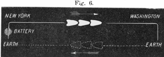
In this case the electric force, necessarily starting from the battery by repulsion, would appear at Washington a certain space of time after leaving New York. And if we should put the opposite pole to the line, we would have the following effect:
