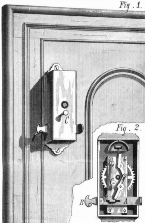
When it is desired to hold the alarm out of action, a pin, C, is pushed inward so as to prevent the movement of the escapement arm.
