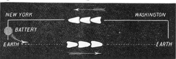
In this case the force would be manifested at Washington by means of the earth connection before appearing at the concavity pole of the battery which is put to the line. All this is assuming that the force is propagated solely by a forward motion or vibration—repulsion.
