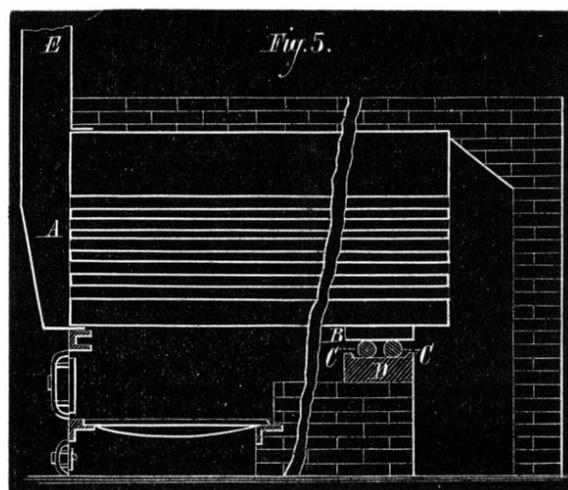
It is obvious that the iron front can be dispensed with, if desired, and the boiler sustained on brickwork alone. This is quite frequently done, but the plan does not appear to possess any special advantages, since, if the setting is properly performed, it will be quite as expensive as if the iron front were used.
