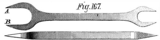
of steel wire flattened out at the ends and filed to the points, A B, the distance between them being the radius of the circle they are intended to scribe or mark. These tools may be used to advantage to mark circles  $\frac{1}{4}$  of an inch and less in diameter, the sizes varying by sixteenths of an inch, and the points being hardened to a brown or straw color.
