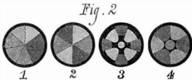
1. Newton's color disk. This consists of seven sectors, red, orange, yellow, green, blue, indigo, and violet respectively. This and the other color disks are made of pieces of stained glass, cemented with Canada balsam to a disk of plate glass, and so admirably fitted that the effect on the screen, even, is of the most perfect finish. Their richness, regularity, and accuracy of color surpass anything which has ever been produced by painting.
