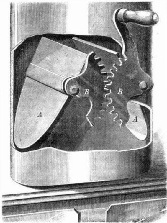
clines thus formed, it is claimed, oppose the draft with less abruptness than the single plate damper, and besides may be more tightly closed than the latter.
