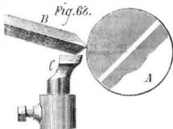
hand rest (the point being used to cut, as shown in Fig. 68, A being the work, B, the graver, and C, the lathe rest), it turns very true and cuts easily and freely. This, therefore, is the position in which it is held to rough out the work.
