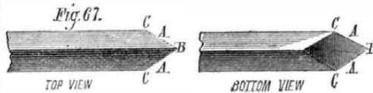
each case a cutting edge, B, the point, and C, in each instance, a heel of the tool. The graver is the most useful of all hand tools used upon metals. It can be applied to either rough out or finish steel, wrought iron, cast iron, brass, copper, or other metal, and will turn work to almost any desired shape. Held with a heel pressed firmly against the
