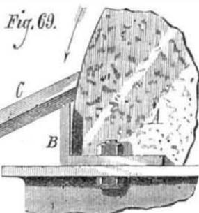
The handle in which the graver is held should be sufficiently long to enable the operator to grasp it with both hands and thus to hold it steadily, even though the work may run very much out of true. For use on wrought iron, the flat
