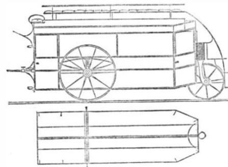
wider and lighter body to be used than in an ordinary omnibus, the total weight of which ranges from 20 to 24 cwt. for 26 passengers; for the same number of passengers, a three-wheeled omnibus might be made to weigh from 14 to 16 cwt. The obvious simplicity of construction makes any technical detailed statement unnecessary, beyond saying that the hind wheel turns round freely in an upright axle box, fitted with a coil spring round the spindle.—*Carriage Builders' Gazette*.
