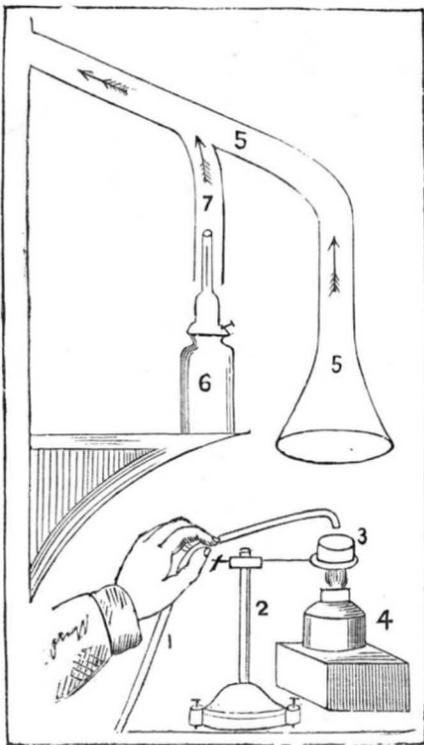
No. 1, a glass tube connecting the gas bag with burners No. 2, an iron stand to hold the small crucible. No. 3, a crucible. No. 4, a small alcohol lamp to ignite the sulphur. No. 5, a funnel to receive the product of combustion. No. 6, a petroleum lamp employed to establish a current of air in the chimney. No. 7, a shaft connected with the chimney, in which the current of air is formed by means of gas or a lamp.
