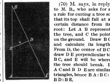
(70) M. says, in reply to M. B., who asks for a rule for cutting a tree so that its top shall fall at a certain distance from its root: Let A B represent the tree, and C the point on the ground. Draw B C and calculate its length. From D, the center of B C, draw D E perpendicular to B C, and E will be where the tree should break. B A C and B D E are similar triangles, hence B A : B C :: B D : B E.
