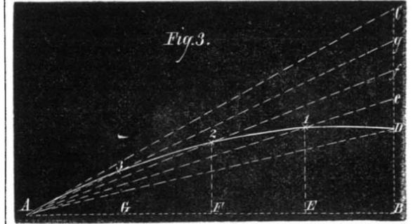
B D is equal to half the sum of the initial and final pitch. Divide C D and A B, each into the same number of equal parts, and mark the points of intersection of lines drawn from the divisions of C D, to A, with the perpendiculars erected at the corresponding points of A B. A curve, D 1 2 3 4 A, drawn through these points and D and A, will be the guide, by means of which the required helix can be traced upon the given cylinder.
