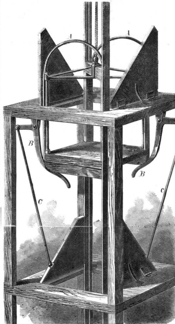
The hatch covers are separated diagonally and are lifted as the car ascends by the curved upper portion, A, of the latter. As the car continues its upward course, the covers are kept raised by means of the bell crank levers, B, connected thereto by rods, C, which levers press against the sides of the car and ease the fall of the doors. In descend-
