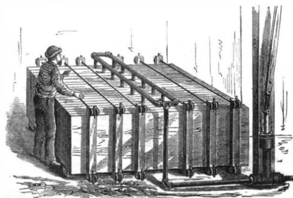
Fig. 4.—PRESSING THE WATER FROM THE SLIP.
