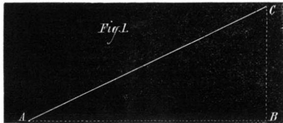
lix, which can be traced on the cylinder by using the edge, A C, of the paper as a guide. If the helix is to be constructed for only a portion of a revolution, make A C equal to that fraction of the circumference, and B C equal to that fraction of the pitch. Similarly, if the helix is to make several revolutions, A B must be the length of the circumference of the cylinder multiplied by that number of revolutions, and B C, the pitch multiplied by the same number.
