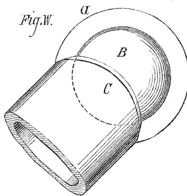
tion, *a* being the chuck, B the ball, and C the cutter.
