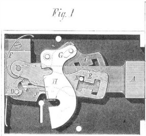
with is that no key, unless specially adapted for performing three distinct functions, namely, the throwing of a main tumbler and guard plates, the bolt, and the latch tumbler,
