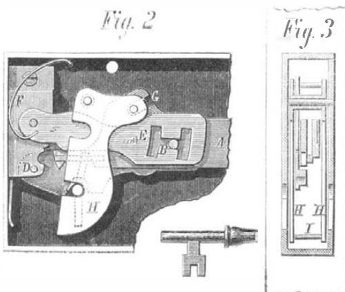
can possibly open it. This will be more evident from the fact that the key holes are closed by guard plates before the motion of the other parts takes place, so that the introduction of implements for throwing the bolt and releasing the tumblers is at once prevented. The action of the key on
