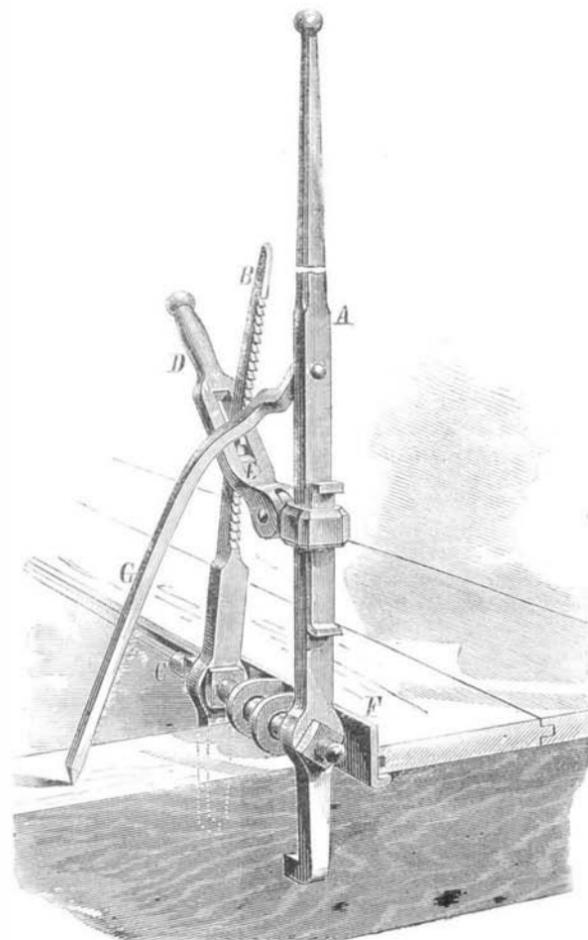
ing to the thickness of the joist. D is the fastening lever, secured, as shown, to the bar, A, and provided with a slot through which passes the bar, B, a step, E, serving to engage in the teeth of and hold the latter at any desired point. F is a plate for protecting the edge of the flooring, and G a pawl for holding the apparatus after clamping up the same.
