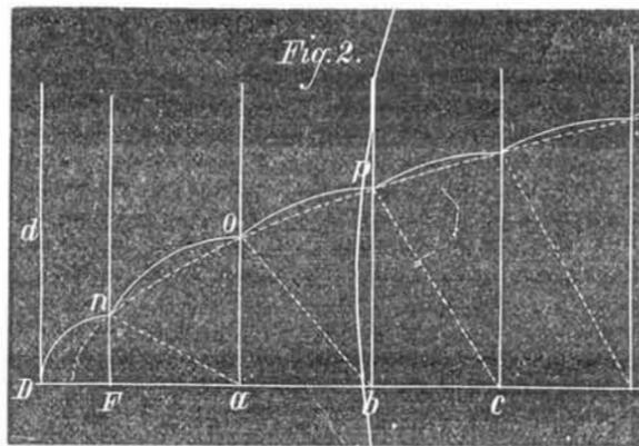
cessary. Then will *n o p* be points in the required curve. Having determined *D F*, and drawn the perpendiculars, *F n*, *a o*, and *b p*, the points *n o p* may be determined without drawing the arcs, by taking the root of every fourth number, beginning with one, from a table of square roots, as shown in the following table, in which  $D F = X$  is taken as the unit.
