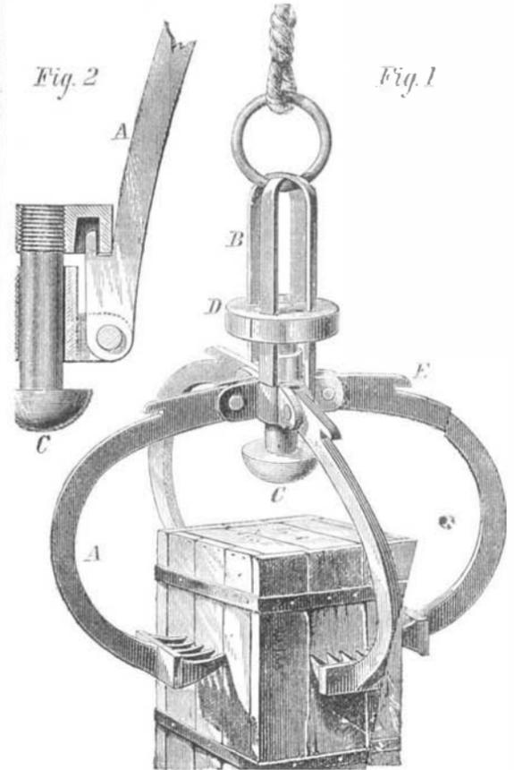
mens of the bottom, in making soundings, the claws may be made scoop-shaped and provided with dis, so that fragments of rock, sand, shell, etc., may be washed away when the apparatus is raised to the surface; or horizontal ribs may be placed upon the arms, when the latter are closed, would form a perfect cage for specimens.
