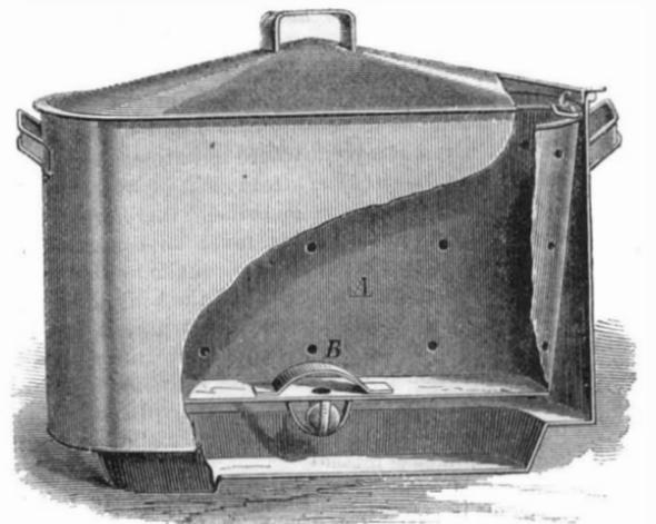
is a ball held in wires or similar contrivances by which its movement is limited. It will be noticed that the inner vessel, A, fits into the boiler steam tight, and that it may be readily lifted in or out, for cleansing or other purposes, by the handles, one of which is shown at C.
