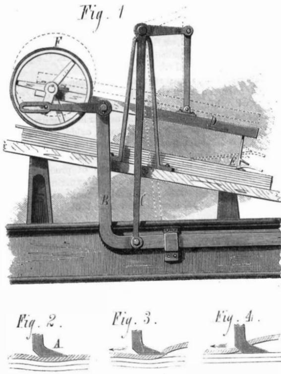
carries the top sheet up with it. At this juncture the grippers come up, seize the projecting edge of the paper, and, drawing the sheet from the pin, carry it down the incline to the press.
