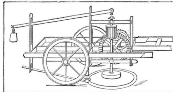
"By the increase of velocity, the scythes revolve with great swiftness. The grass, as it is cut, is first thrown by the progressive motion against a rise in the scythe frame toward the center, and by the same motion is afterwards thrown off in a regular row, following the center of the machine."
