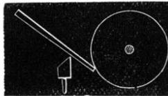
should be placed a little below the center of the wheel, and the iron held as in the figure. The wheel of course runs towards the operator. The theory of the operation seems to be that the particles of emery become imbedded in the iron and then react on those still remaining in the wheel, on the same principle that diamond dust on a soft wheel is employed in cutting diamonds.
