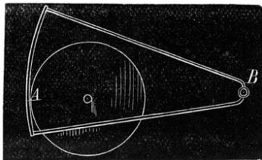
A, which receives a vibratory motion on its axis, B, by suitable mechanism, and the stone revolves against it, having, in addition, a sidewise motion imparted, so that it travels across the face of the saw, making it wholly equal in all parts.
