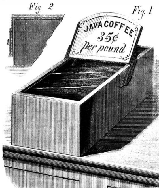
Fig. 2. An inclined plate is arranged with projecting arms, which enter sockets on either sides of the box, and serves to support a card suitably inscribed with name, price, or other information.
