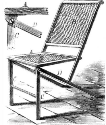
back which extend below the seat, act as hind legs for the support of the seat when the chair is extended. The inclination of the back and seat can be varied, for which purpose notches are cut in the bars, D. It will be understood, from the illustration, that the chair, when not in use, can be folded up into a very small compass.
