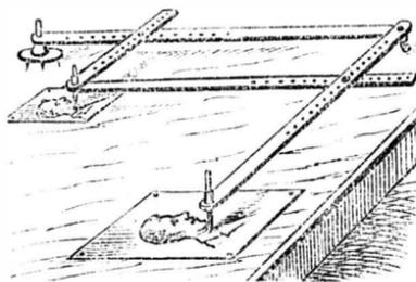
shows its operation more clearly. The apparatus is very easily constructed from wood or metal. Some care should be taken in making the joints, in order that they may work very easily without shaking.
