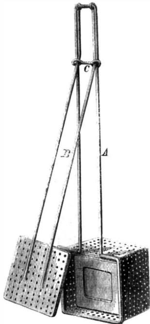
When closed, with the soap on the inside, the box is dipped in the water and shaken until the requisite lather is obtained. It is then removed and placed upon the washstand. This device was patented through the Scientific American Patent Agency, May 7, 1872, and is the invention of Mr. Jacob A. Camp, of Sandusky, Ohio.
