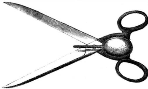
the sides of the rubber ball and hold it in position, while the ball, by its elasticity, forces apart the handles and opens the blades. The inventor claims that the improvement can be advantageously attached to shears for other than barbers' use.
