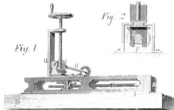
screw immovably affixed to the head block. D is a sleeve nut traversing said screw, and connected with the knee by means of the stirrup, E, as more clearly shown in the sectional view, Fig. 2. The same engraving represents how the edges of the horizontal portion of the knee, B, are grooved to slide in a slot in the upper portion of the head block.
