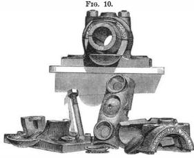
(Fig. 10). The box is furnished with spherical surfaces to fit in sockets in the casting or frame; it is self-adjusting as to line, but cannot be raised or lowered as in the case of the hanger. It takes the place of what is known as the clamp box, and of any rigid bearing not adjustable. It was a clamp box that I found among the many ingenious illustrations of mechanical devices in the cabinet in the room of your Professor of Mechanical Engineering. I have it here (Fig. 11).
