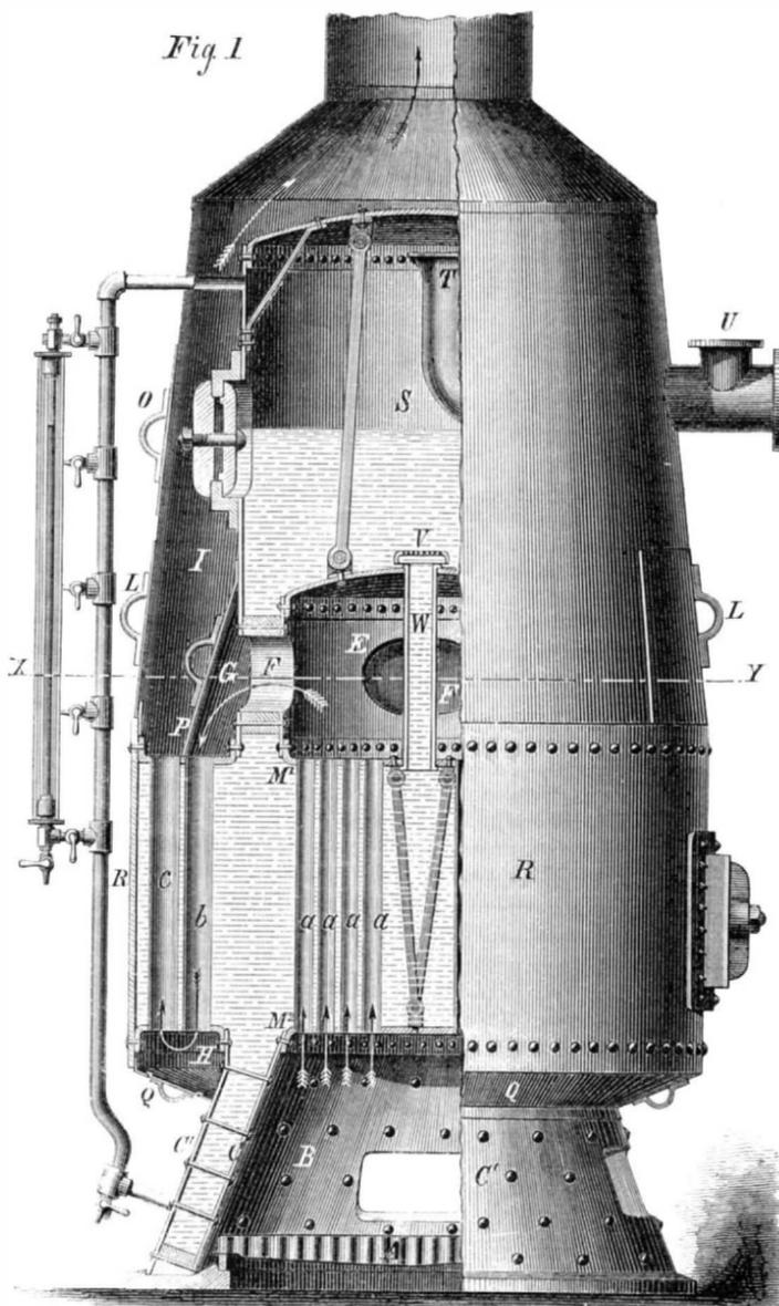
products of combustion following the direction of the arrows in the engraving, arising from B, first pass through the fire tubes, a a a, into the mixing chamber, E. From this receptacle, the gases have their exit through the large openings, F F F, and after having imparted a portion of their heat in the ordinary manner, are retained by the conical casing, P, which incloses the space, G. They are consequent-
