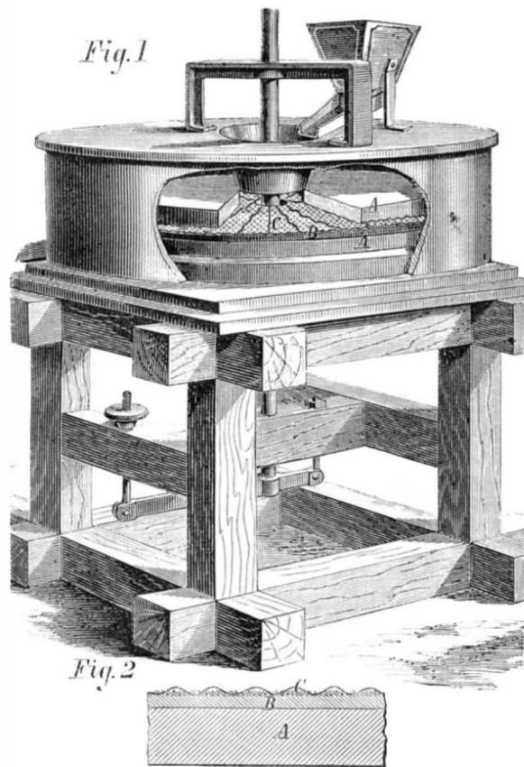
It will be seen from Fig. 1, which represents the machine with part of the cover and one of the stones broken away to show the interior parts, that it is similar in construction to an ordinary grain mill. At A are the two polishing or hulling stones in blocks. The polisher, A, is shown also in Fig. 2 which is a detail section of the same.
