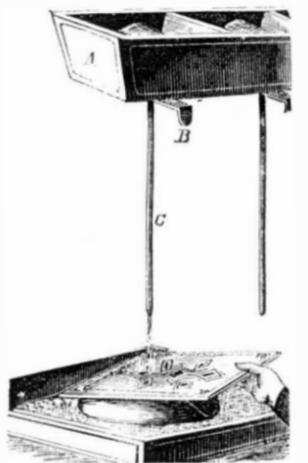
As fast as the supply of engraving powder runs down through the tube, it is replaced in the hopper; and girls may do all the work. That portion of the articles that is not to be engraved is protected by paper or other substance. The engraving, therefore, is done by cutting out the desired pattern in paper, which is then applied to the surface of the article. The powder only acts between the interstices of the pattern.
