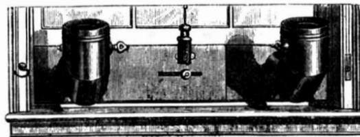
Short sheet metal elbowed tubes are fixed in pieces of board, which overlap and are held together by a bolt which passes through a slot in one of them, so that they can be adjusted to fit windows of different widths. These boards are placed with their outer ends flush to the window casing, and the lower sash is raised to rest upon the upper edge of the apparatus. The joints are made tight with suitable packing. Each elbow tube has a damper to regulate the admission of air.
