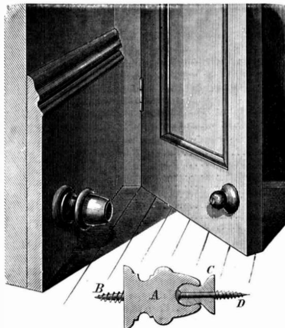
thrown open, and at the same time to keep the doors in the open position when so desired. The objection to devices now in use, for overcoming the concussion in throwing the door against the washboard pedestal, is the rebound they give the door, throwing it away from the position designed for it. To obviate this, several devices have been brought out, consisting of springs, ratchets, catches, etc., most of which have been proved too intricate and expensive for the purpose.
