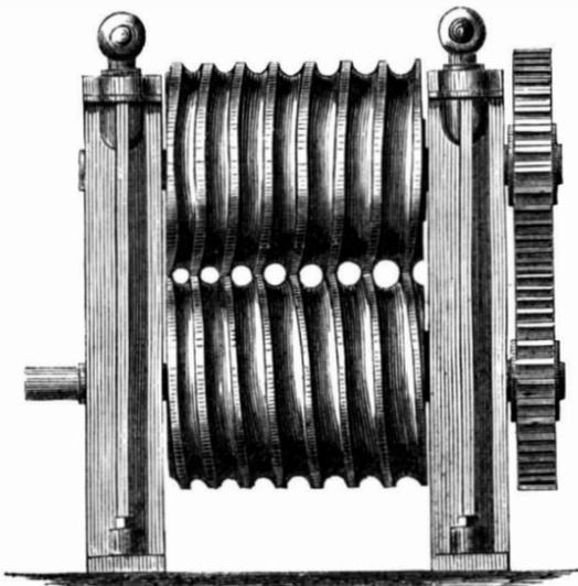
gether and geared, so as to revolve in union, the grooves form a series of eyes, which, as the rolls revolve, appear to move laterally, and gradually decrease in size. Thus, if a bar or tapered strip of iron, bent so as to approximately form a tube, be introduced between the rolls at that end where the grooves are largest and deepest, it will be gradually shifted towards the other end of the rolls as it passes between the latter, and will thus be rolled tapered.
