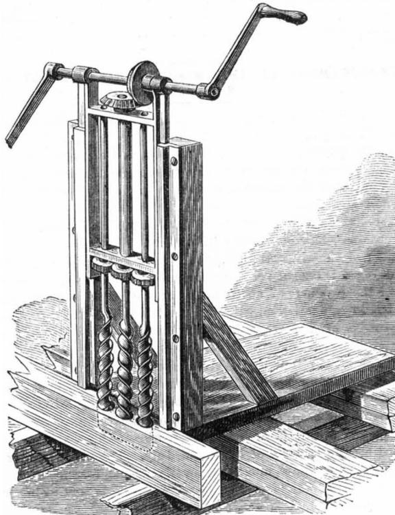
single one. The power is first transmitted to the central auger, and from its shaft to the others by means of gearing, the two outside ones having their twist and cutting edges in the opposite direction from the middle one.
