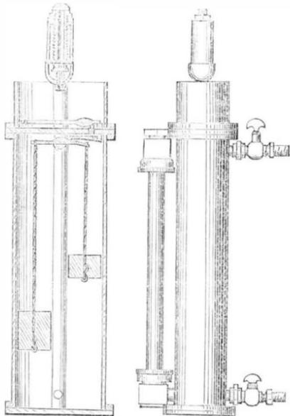
of the large stone, the difference in the weight, operating on a cam lever and a supplementary lever, will raise the safety valve, and admit the steam to the whistle. If water be again pumped into the boiler, and raised high enough to submerge both stones or weights, the gravity of the weights becomes relatively what it would be if both were out of the water, again raising the valve and giving the alarm, either of these causes being determined by inspecting the glass gage.
