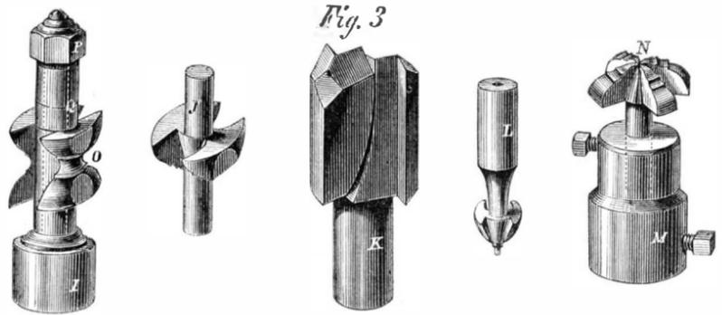
molding, and grooved, by the cutter, K, Fig. 3, on the other, as shown by dotted lines, to receive the seat and back.
