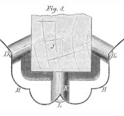
Fig. 3 is a section of flooring and metallic ceiling for manufactories. etc., in which the letters H represent, respectively, Our readers will be prepared, by several articles which a metallic arch with rib moldings, and also a metallic arch to support the concrete underneath the flooring ; J the joists, and C the flooring.
