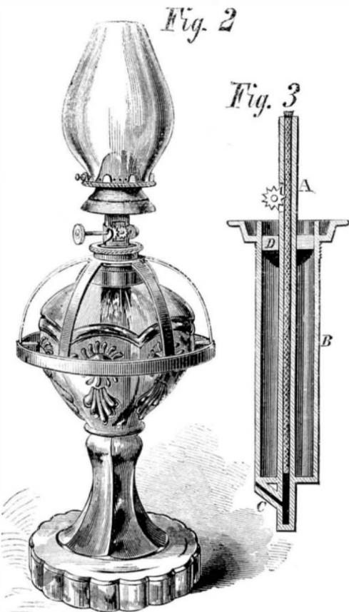
The reservoir, A, is of polished metal, so as not to absorb the heat rapidly, and is closed by a screw cap. The wick tubes, B, are about three inches from the lamp, supported by braces, as seen; on the lower ones of which rest the pipes, C, which convey the oil to the wicks. The burners are of the usual form. The distance between the flame and the reser-
