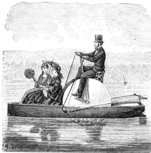
by two cords passing from the steering bar, over pulleys fixed upon the side of the boat below and in front of the operator, and from thence back to the tiller.
