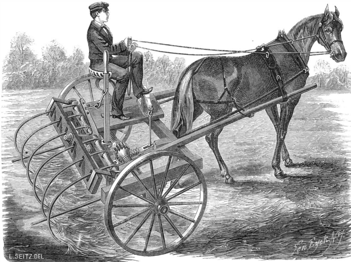
HUNSBERGER'S PATENT SELF-DISCHARGING HORSE RAKE.
