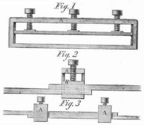
ing to the width of the belt, the sizes of the clamps or coupling being adapted to the different widths of belts. Its meth od of application is shown plainly in Figs. 2 and 3.
