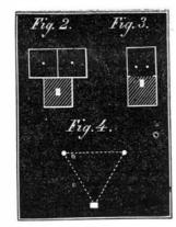
produced in the one tube, O, there are exactly two measures of hydrogen evolved in the tube, H. Water is by this experiment proved to consist of oxygen and hydrogen in the pro portion of one measure of the former to two measures of the latter. This has been represented in Fig. 2, where each measure is represented by an equal square, and H standing for hydrogen, O for oxygen.
