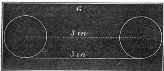
G. Roll it 3 inches over a right line, and the path of the axis will be 3 inches. Then 3 divided by 3 equals 1 revolution on its axis.
