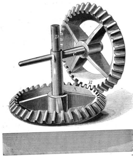
Here we have a fixed wheel, A, and a movable wheel, B, of the same diameter; and we say that the moving wheel turns *once on its own axis* in rolling once around the fixed wheel. We should be glad if the two-revolution philosophers would examine and tell us explicitly, whether, in the above example, the moving wheel makes *one* or *two* revolutions upon its own axis, in rolling once around the fixed wheel.
