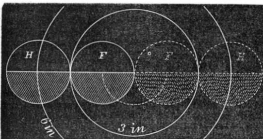
H. Roll it once around the convex surface of a wheel of same size, and the path of its axis will measure 6 inches. Then 6 divided by 3, equals 2 revolutions around its own axis.
