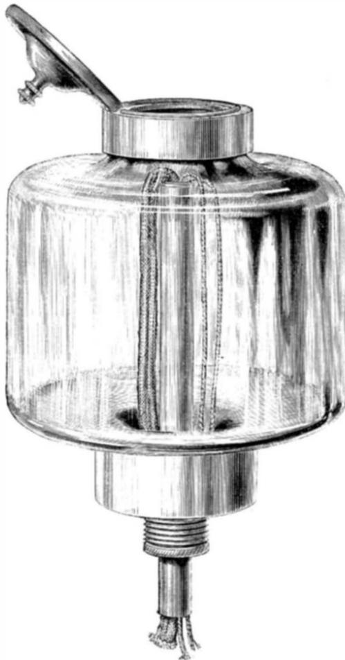
to the journal by capillary attraction. Much practice is necessary to adjust the size of this wick to the amount of oil it is desired to deliver, which depends on the size and velocity of the shaft journal, weight, etc. If the wick fits too tight or the oil gets too low the supply of the lubricant is diminished, while if the wick is loose or the cup too full the amount delivered is too large. The cups, in fact, act on the principle of gravitation as well as of capillary attraction.
