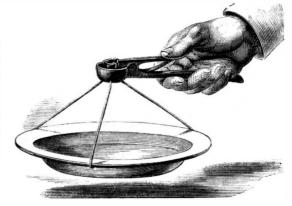
are bent into hooks at their outer ends. The long end of the lever is kept up by a curved spring except when depressed by the thumb, The engraving shows plainly the manner of using. The wires are placed over the rim of a plate—being spread to their full extent by the spring—when the thumb presses the lever down contracting the hooks toward the center and holding the plate firmly.
