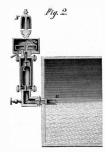
This alarm device consists of the single valve, L, whereby the orifice of pipe, M, is kept closed as long as the water stands above the dotted line, but is opened as soon as the wafalls below the line, to allow the steam to flow through pipe, M, for the purpose of blowing an alarm whistle, N. The apparatus is represented in Fig. 2 in the state of allowing the steam to flow through it, for the purpose of blowing a whistle.
