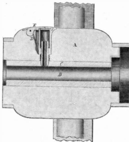
moving the wheels; one that will keep out the dust and still be adapted to every size of hub by simple adjustment. It is a tube formed in two parts, one to slide or be screwed within the other to adapt its length to hubs of varying diameters.
