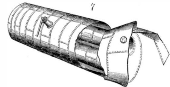
the outside of this flue must be immense, and it had no other resistance to offer but its cylindrical form and the strength of the material. Internal tubes, when of large diameter and used for flues, should be as capable of resisting external force as the shell of resisting internal strain. A convenient way of strengthening these flues is by rings. They may be of T-iron, or of plate iron the central portion rolled into a curved form
