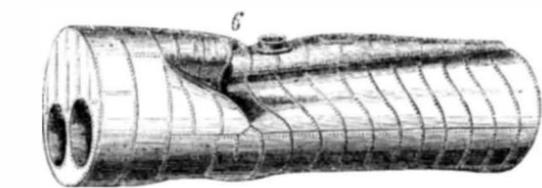
The boiler represented in the engraving was thirty-four feet long and five feet six inches diameter.
