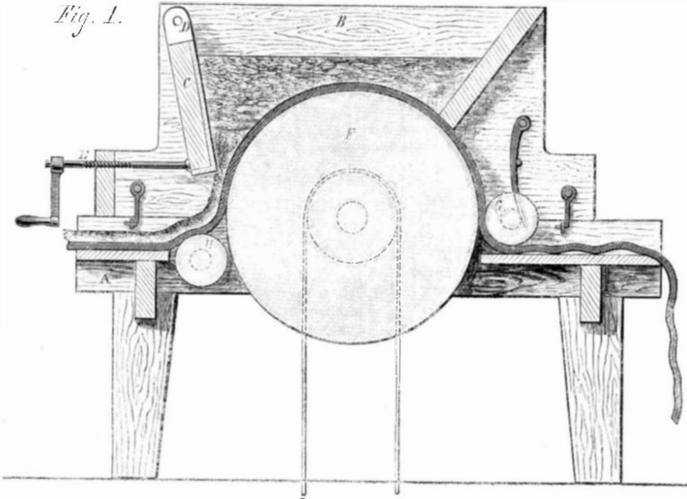
**PULTE'S CEMENT-SPREADING MACHINE.**
