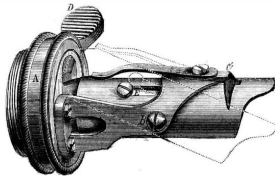
held, in the act of charging, directly over the muzzle. But with the charger shown in the engraving neither the hand nor the flask is held in range of the barrel, and if the powder from the charger should prematurely explode, it will not ignite that in the flask, as the communication between the two is closed.
