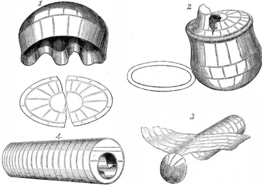
surely cut the angle iron around the rim. In the latter case corrosion might have caused the rupture, as the joint between the bottom and sides appears to have been left intact.
