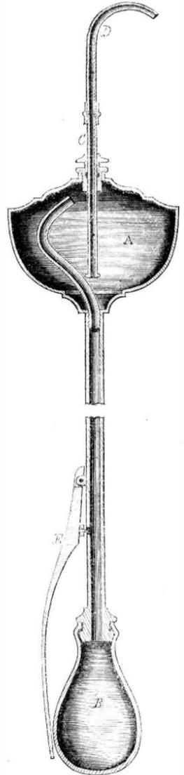
The operation is as follows:—In oiling overhead the curved nozzle is attached to the discharge pipe, which is pushed down to near the bottom of the reservoir. In the action of compressing the bulb, the handle of the lever, E, is depressed which closes the side hole in the pipe and makes it air tight. The air thus forced into the reservoir presses upon the surface of the oil and ejects it through the nozzle, D.
