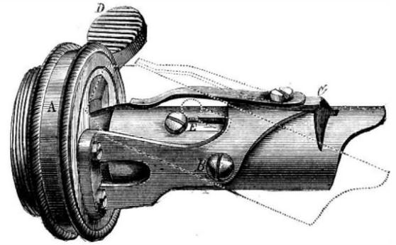
held, in the act of charging, directly over the muzzle. But with the charger shown in the engraving neither the hand nor the flask is held in range of the barrel, and if the powder from the charger should prematurely explode, it will not ignite that in the flask, as the communication between the two is closed.
