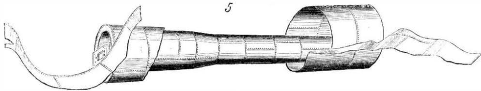
extends to the sound seam beyond the bridge wall and in front to the head, and then runs up the transverse seams at either end of the longitudinal rent, opening the shell out on either side. Sometimes, however, the head blows off and the body of the boiler is thrown violently from its bed. This is often the case where the heads are of cast iron flat; or, the portion nearest the fire is torn without regard to the seams.
