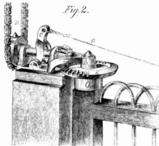
resting upon the two forward rollers and the hind bolster. The chains, C C, in connection with the crank and shaft are used to bind the load and also in connection with the ropes and hooks connecting the two hind pairs of stakes to move backward the forward pair, and forward the hind pair, which motion raises all the rollers from the frame and discharges the load, leaving it in a compact pile and without breakage or damage to lumber.
